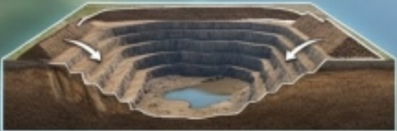
Slag relocated to fortify walls
